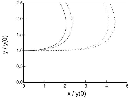
**Figure 3.** A comparison of the compacted and uncompactd normalized Ernst profiles in two different cases: (—), compacted profile,  $r = 1$ ; (---), uncompactd profile,  $r = 1$ ; (·····), compacted profile,  $r = 3$ ; and (-·-·-), uncompactd,  $r = 3$ .
