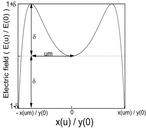
**Figure 2.** The general form of the normalized electrical field in the compacted Ernst-like profile.
